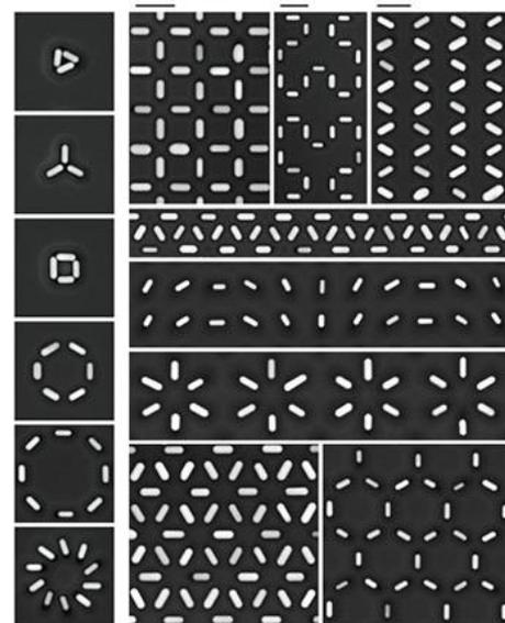
**Examples of two-dimensional patterns of Au nanorods fabricated by topographically templated capillary assembly (scalebars: 250nm)**
