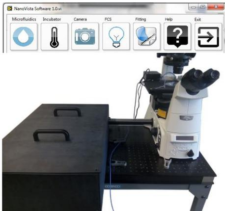
FCS accessory for inverted microscopes manufactured by COSINGO
