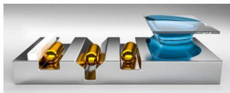
**A solvent drop is dragged over a patterned template and the particles assemble in the grooves**
