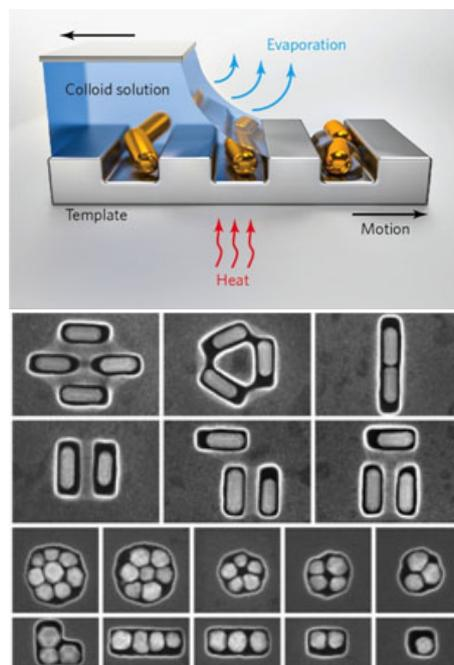
Fig. A solvent drop is dragged over a patterned template and the particles assemble in the grooves.
