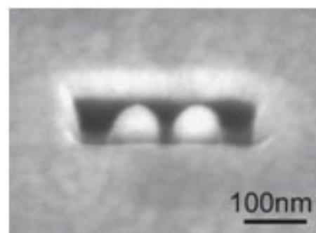
Fig. SEM image of a fabricated nano “antenna-in-a-box”.
