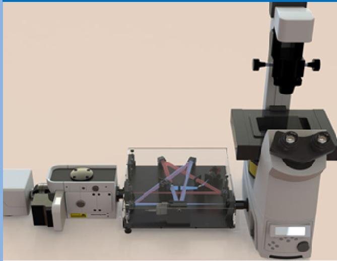
Our first NEXPRESSO Type 1 project has finished. Using a component supplied by Cosingo - Imagine Optic, the Institut Curie worked on a project called "Adaptive Optics in Spinning Disk microscopy (AOSD) of living samples". The aim was take advantage of adaptive optics (AO) to correct for sample and system induced aberrations. AO would be integrated into fast multi-focal microscopy at very low S/N ratio, for observation on live "medium thick" biological samples.
